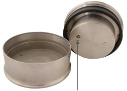
Adjusting screw for calibrating the barometer.
